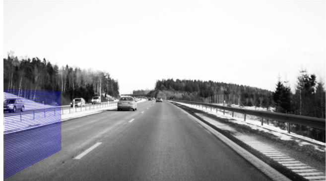
Fig. 1: Overview of the idea. 1D feature points are detected and tracked along so called detection lines (blue lines to the left). The slope of these lines are such that they intersect in the vanishing point, meaning that an overtaking vehicle is moving along these lines.
